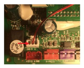
Replace it by cable with proper grounding (GND) included in kit:
