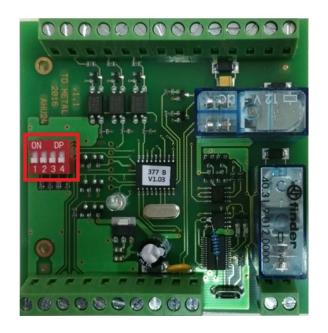
There are 16 positions of DIP slides, corresponding to 0-90% capacity of compressor via 6% steps. Please, set demanded fix capacity using manual slides per schematic diagram below.
